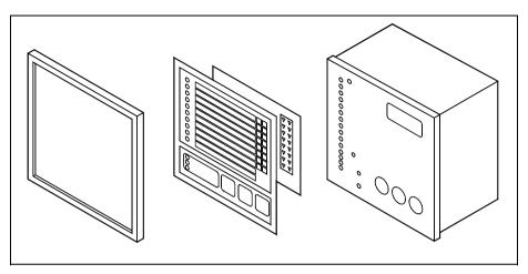
The descriptive text for alarm channels 1-8 and the output channels A and B is written/set on the shown text label.
